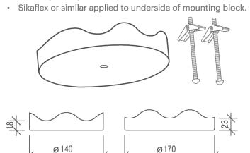
RECOMMENDED ARCPANEL FIXING FOR CABLE TRAY
