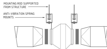
**IN-LINE-CENTRIFUGAL FAN MOUNTING DETAIL**
