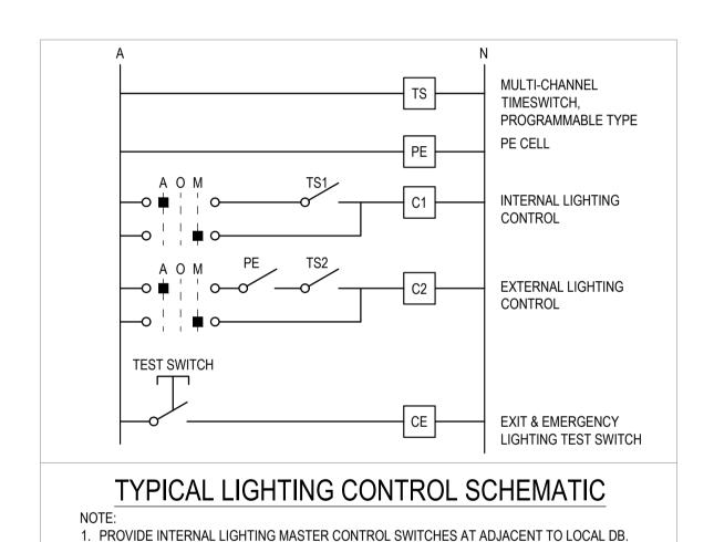
2. PROVIDE EXTERNAL LIGHTING MASTER CONTROL SWITCHES AT ADJACENT TO LOCAL DB.
