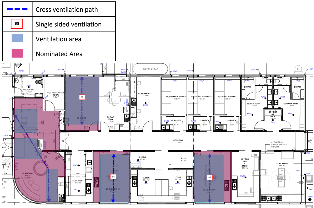
Figure 4: Natural ventilation assessment
