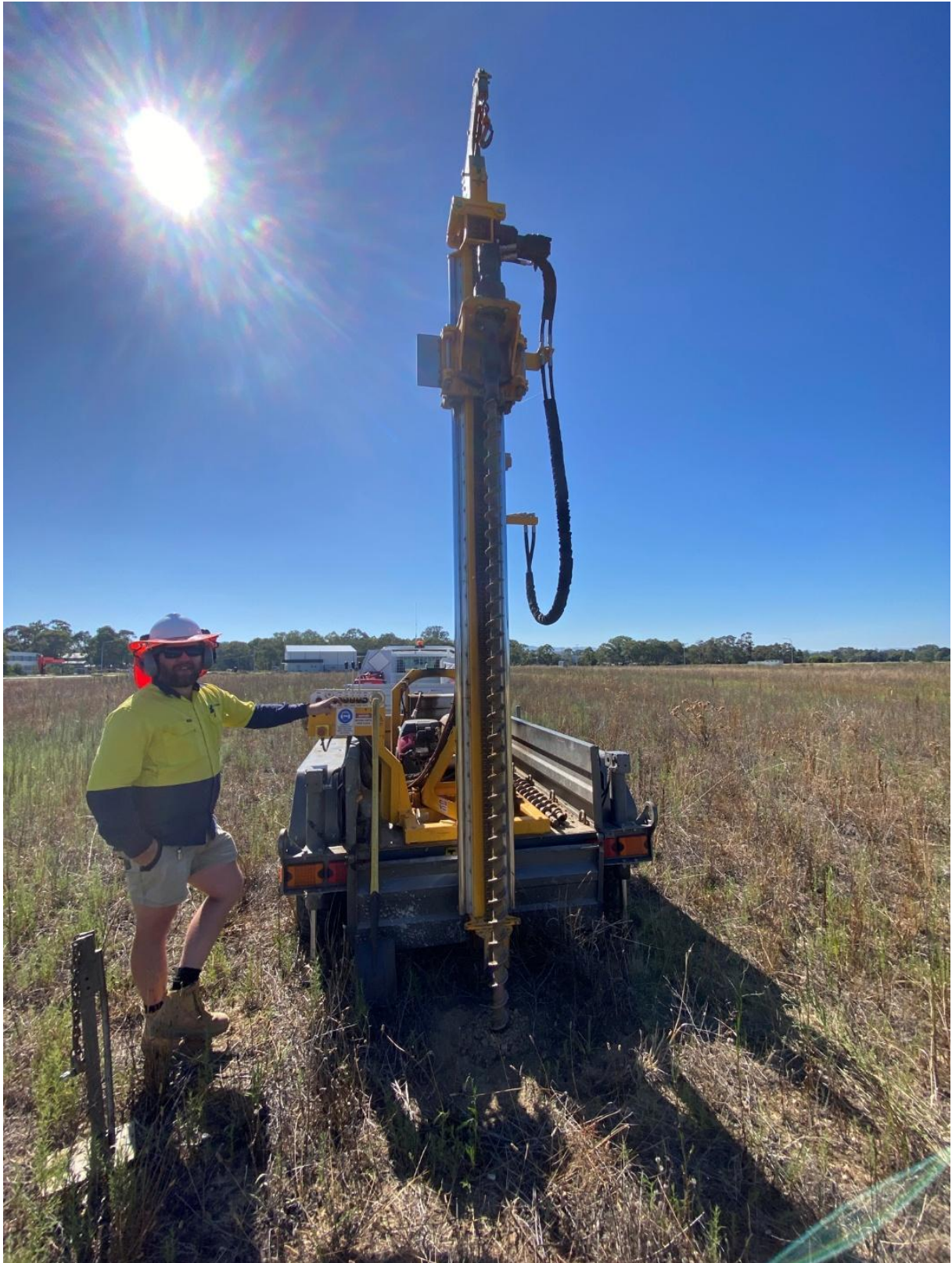
Photograph 3: The sampling method used on site – Power auger.
